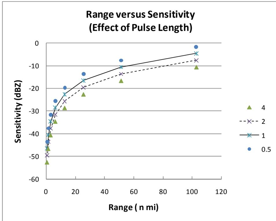
Figure 13. Range versus sensitivity for the Radtec 43/250 for pulse lengths of 4, 2, 1, and 0.5 microseconds.
