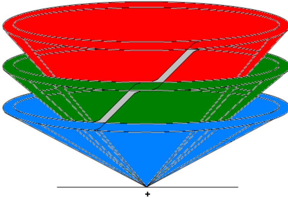
Figure 3. A 3-D schematic representing the radar coverage by provided by three 360° scans with antenna elevation changes shown as grey ramps.
