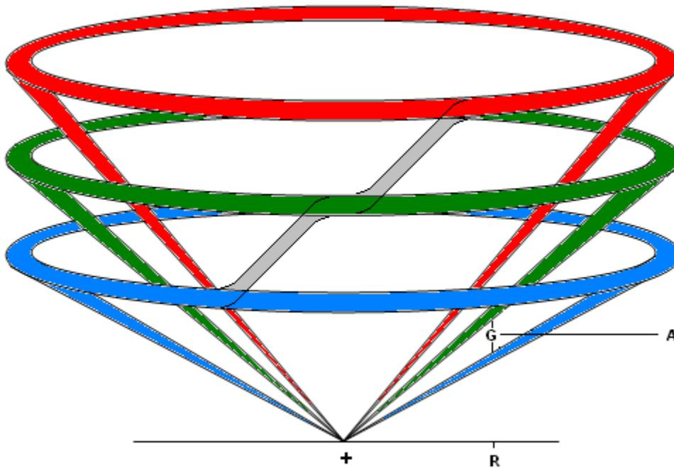
Figure 5. A schematic of radar beams from adjacent elevation angles. The vertical gap  $G$  is shown at range  $R$  and altitude  $A$ .
